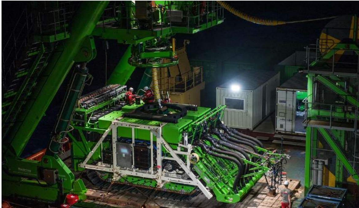
Figure II- 6: Photograph of the pre-prototype vehicle (PPV) Patania II and associated Launch and Recovery System, developed and built by GSR.
