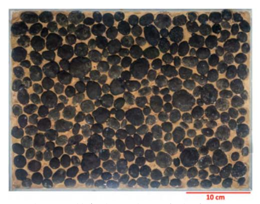
Fig.4. Test section, with 286 Type 1 nodules from the NORI exploration site (≈ 16 kg ww)
