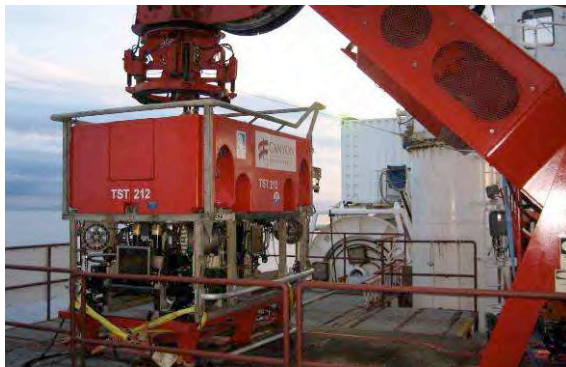
Plate 1. The Mercury Wave, the remote operating vehicle (ROV) and lowering of ROV to water using the crane at rear of boat
