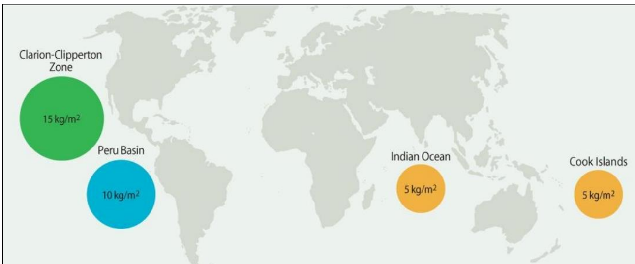
Figure 6.1 Schematic diagram of average abundance of polymetallic nodules in four major locations
