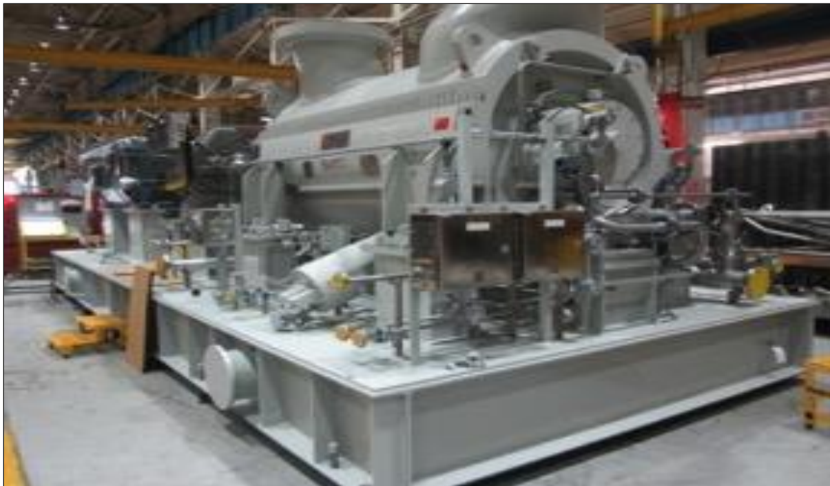
Figure 13.15 Main air compressor (Elliott Group model 46M6I)
