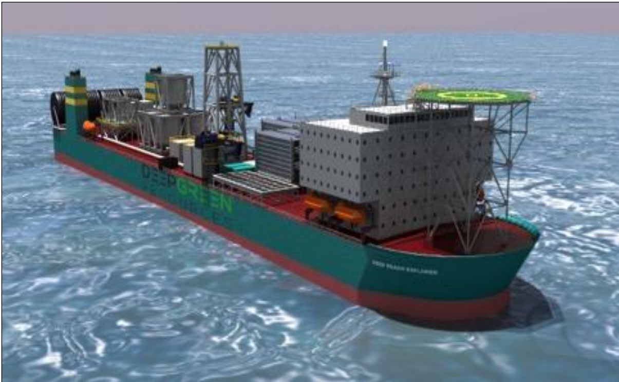
Figure 13.10 Collector Ship 1, production support vessel
