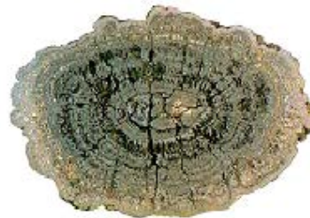
Cross-section of manganese nodule
