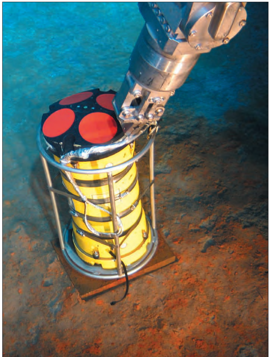
Plate 7.5 300 kHz ADCP current meter deployed by ROV on the Solwara 1 mound
