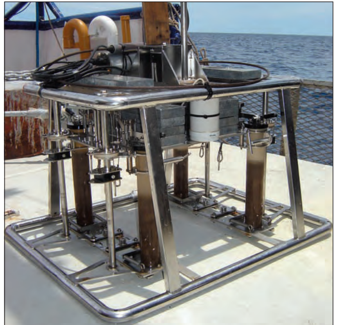
Plate 7.24 Sediment samples taken on the abyssal plain 10 km west of Solwara 1 using multicorer
